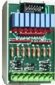
Passive interface module with 8 inputs for connection of electronic instruments, PLC and various interfaces.
